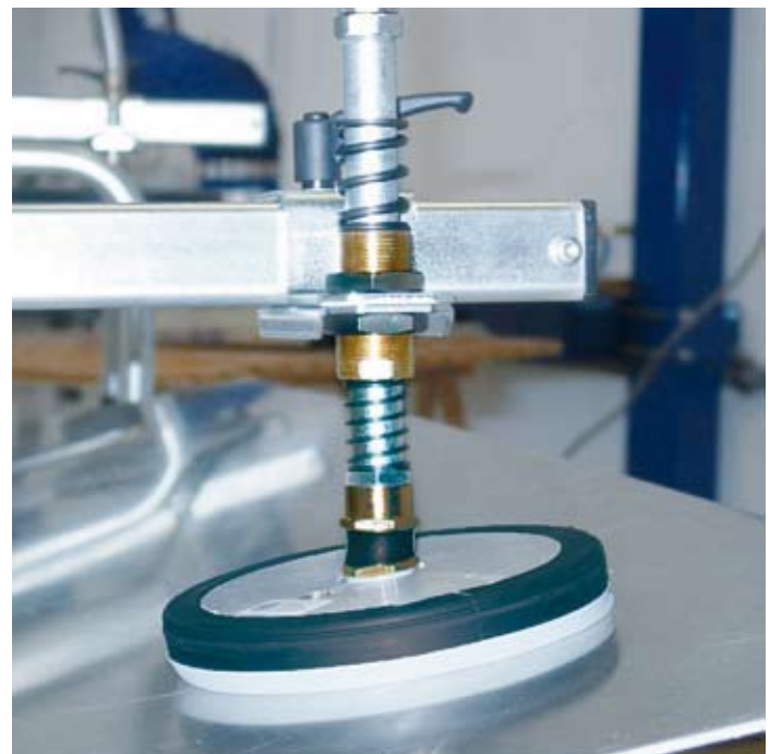
Suction gripper with spring-loaded plunger and angle joint mounting for angled support of workpieces
