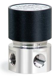
TESCOM BB-3 is a high pressure, low flow, miniature backpressure regulator. Six control pressure ranges are available up to 1200 psig / 83 bar outlet. This regulator can be used for hydraulic or pneumatic service and is small and compact, weighing approximately 4 oz / 0.11 kg in the standard Aluminum construction (316 Stainless Steel also available).
