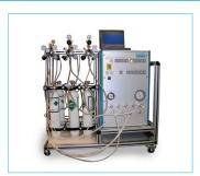
APT-Automated Performance Tester provides a test gas sequence for automotive exhaust analyzers to check the entire gas sampling path.
