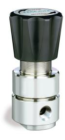
TESCOM 44-2200 Series is a compact, lightweight high purity single-stage regulator for specialty, flammable, and industrial gas flows of less than 5 SCFM / 141 SLPM. Its diffusion-resistant metal diaphragm seal ensures gas purity and integrity.
