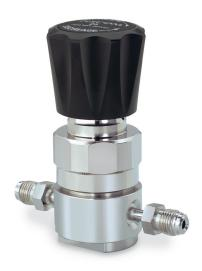
TESCOM 64-2600 Series economical high purity pressure reducing regulator provides Stainless Steel construction with 10 R<sub>a</sub> surface finish and is electronic grade cleaned. Inlet pressures are 600 or 3500 psig / 41.4 or 241 bar with outlet pressures of up to 250 psiq / 17.2 bar.
