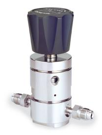
TESCOM 64-5000 Series ultra high purity, absolute/subatmospheric pressure reducing regulator offers a 10 R<sub>a</sub> surface finish. Inlet pressures are 120, 600, or 3500 psig / 8.3, 41.4, or 241 bar with outlet pressures ranges from 50 mm Hg absolute - 15 to 100 psig / 50 mm Hg absolute - 1.0 to 6.9 bar.
