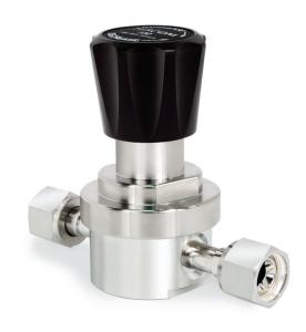
TESCOM 22-5400 Series high purity, high flow BA Grade pressure reducing regulator offers a C<sub>V</sub> = 1.0 and a 316 Stainless Steel Electropolished body of 25 R<sub>a</sub>. Inlet pressure is 600 psig / 41.4 bar with outlet pressures up to 150 psig / 10.3 bar.
