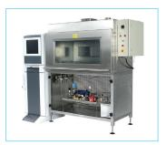
Test bench allows accurate hydrostatic testing of car radiator hoses according to DIN EN ISO 1402 European standard. Inspects initial samples and randomly tests hoses during ongoing production.
