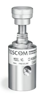
TESCOM CC Series metering valve is rated to 10,000 psiq / 690 bar and contains a non-rotating stem to reduce seat and stem wear. The valve features over 20 turns from shutoff to full open, providing excellent flow control.
