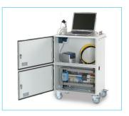
Mobile test rig monitors medical systems in hospitals. Pressure, flow capacity and leakage demands are verified.
