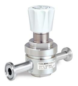
TESCOM PH-3200 Series is part of our Pharmpure™ product line. This high purity high flow singlestage regulator offers a compact, USP Class VI and BPE compliant design suitable for biotech and pharmaceutical applications. This regulator offers gas flows of 5-50 SCFM / 142-1416 SLPM. Diffusion-resistant metal-to-metal diaphragm seal ensures gas purity and integrity.
