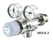
TESCOM single-stage WEGA 1 and dual-stage WEGA 2 cylinder pressure regulators are for gas purities up to 6.0 quality. A relief valve is integrated into the body for low internal gas volume. Both models are lightweight with a compact design.
