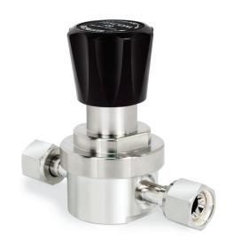
TESCOM 64-5400 Series high purity pressure reducing regulator provides 316 Stainless Steel with Electropolish, 10 R<sub>a</sub> surface finish and Hastelloy® diaphragm design. The 64-5400 Series offers high flow  $C_V = 1.0$  and inlet pressure of 600 psig / 41.4 bar with outlet pressures up to 150 psig / 10.3 bar.
