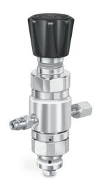
TESCOM 64-3400 Series dual-stage, ultra high purity pressure reducing regulator offers a tied diaphragm design and 10 R<sub>a</sub> microinch / 0.25 micrometer surface finish with optional Hastelloy® trim. Inlet pressure is 3500 psig / 241 bar with outlet pressures up to 150 psiq / 10.3 bar.
