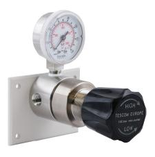
TESCOM High Pressure Point-of-Use regulator is a 44-1800 Series pressure reducing regulator that is spring loaded, hand operated and piston sensed.
