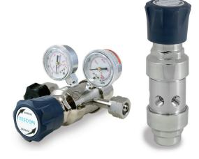
TESCOM SG2 Series is a compact, lightweight, high purity two-stage cylinder regulator for specialty, flammable and industrial gases. Sensitive, extra long-life metal diaphragm ensures gas purity and integrity. User-friendly model number enables the specifier to select optional gauges, relief and shut-off valves, and cylinder connections as part of the regulator assembly.
