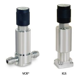
TESCOM 12 Series is a miniature ultra high purity IGS/VCR pressure reducing regulator. The 12 Series offers 5  $R_a$  or 10  $R_a$  microinch finishes, tied diaphragm and internally springless and threadless design. It provides inlet pressures of 150 psig / 10.3 bar, outlet pressure from 250 mm Hg-15, 30, 60, 100 psig / 250 mm Hg-1.0, 2.1, 4.1, 6.9 bar with flow rates up to 120 SLPM.
