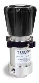
TESCOM 26-1000 Series controls pressures up to 10,000 psig / 690 bar. This pressure reducing regulator offers standard venting providing decreased outlet pressure. The 26-1000 Series has an interchangeable spring and sensor for product versatility. The low torque handknob is easy to adjust.
