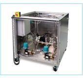
Test stand allows hydrostatic durability and leak test up to 60,000 psiq / 4000 bar.
