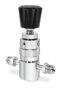
TESCOM 449-254 Series high purity, high flow pressure reducing regulators are ideal for high pressure bulk specialty gas delivery systems (BSGS). The 449-254 Series offers a  $C_V = 1.0$ , surface finish of 10 R<sub>a</sub> and is available with Hastelloy® trim. Inlet pressure is 1500 psiq / 103 bar with outlet pressures up to 400 psig / 27.6 bar.
