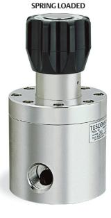
TESCOM 26-2500 Series has a  $C_V$  = 5.0 for high flow backpressure applications. Large diaphragm provides excellent sensitivity and minimal crack-to-reseat pressure differential.
