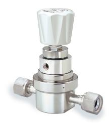
TESCOM 74-3800 Series ultra high purity, tied diaphragm pressure reducing regulator offers high flow and internally threadless and low internal volume design with  $C_V = 0.5$ . The 74-3800 Series is available with 10 R<sub>a</sub> surface finish. Inlet pressures are 600, 1000, or 3500 psiq / 41.3, 69, 241 bar with outlet pressures up to 150 psiq / 10.3 bar.
