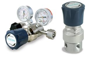
TESCOM SG1 Series is a compact, lightweight high purity single-stage regulator for specialty and industrial gases. Sensitive, extra long-life metal diaphragm ensures gas purity and integrity. Userfriendly model number enables the specifier to select optional gauges, relief and shut-off valves, and cylinder connections as part of the regulator assembly.
