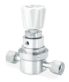
TESCOM 23 Series ultra high purity in-line regulator offers 10 R<sub>a</sub> microinch finish with high flow capabilities up to 950 SLPM. The tied diaphragm 23 Series provides an internally springless and threadless design with inlet pressure of 250 psig / 17.2 bar and outlet pressure up to 100 psig / 6.9 bar.
