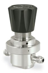
TESCOM 64-3600 Series ultra high purity, highly sensitive pressure reducing regulator offers a low droop, tied diaphragm design, 10 Ra / 0.25 micrometer surface finish with available Hastelloy® trim. Inlet pressures are 600 or 3500 psig / 41.4 or 241 bar with outlet pressure up to 150 psig / 10.3 bar.
