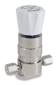
TESCOM 74-2400 Series ultra high purity, tied diaphragm pressure reducing regulator provides low internal volume and an internally springless and threadless design. The 74-2400 Series offers a 10  $R_{\mbox{\scriptsize A}}$  surface finish and 316 Stainless Steel VAR. Inlet pressures are 600 or 3500 psig / 41.3 or 241 bar with outlet pressures up to 100 psig / 6.9 bar.
