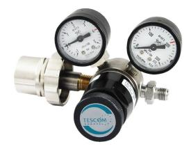
TESCOM WEGA Mini is a cylinder pressure reducer for gas purities up to 6.0 (99.9999 Vol %) used for lecture bottle and mobile applications. Lightweight and compact design due to the relief valve integrated into the body.
