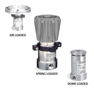
TESCOM 54-2100 Series backpressure regulator is suitable for 15,000 psiq / 1034 bar liquid applications. Modifications are also available for 20,000 psig / 1379 bar and 30,000 psig / 2068 bar. Hardened Stainless Steel seat and stem provide excellent wear resistance in harsh applications.
