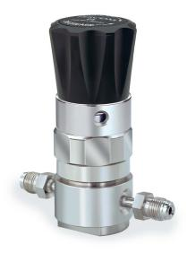
TESCOM 64-2800 Series high purity, tied diaphragm pressure reducing regulator offers Stainless Steel construction with 10 Ra microinch / 0.25 micrometer surface finish and is electronic grade cleaned. Inlet pressures of 1000 or 3500 psig / 69.0 or 241 bar with outlet pressures up to 150 psig / 10.3 bar.
