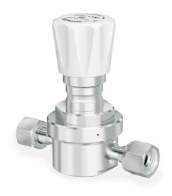
TESCOM 74-3000 Series ultra high purity pressure reducing regulator offers 5  $R_a$  or 10  $R_a$  surface finishes, high flow  $C_V$  = 0.5 and an internally threadless and low internal volume design. Inlet pressures are 600, 1000, or 3500 psig / 41.3, 69, or 241 bar with outlet pressures up to 150 psig / 10.3 bar.
