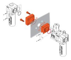
Panel adapters are available to enable air preparation products to be easily mounted inside or outside the enclosure. No additional piping is required and because the enclosure does not need to be opened to shut off the pneumatic air supply, this improves safety.
