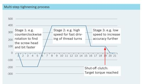
Stages 1, 2 (and 4) can be activated as required. Stage 3 is the standard stage in which the speed can be set between 50 and 100% as required.
