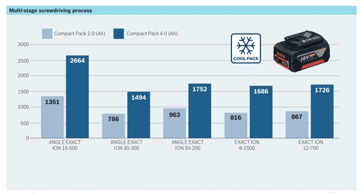
Results of endurance test 02/2013, at maximum torque and a medium-hard screwdriving application at  $80^{\circ}$  rotation angle, measured from a threshold torque of 50%, at screw size M8
