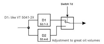
Fig. 33: Adjustment to the connected oil volume
