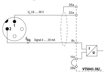
Fig. 23: Connection pattern for pressure transducer HM20...C...
