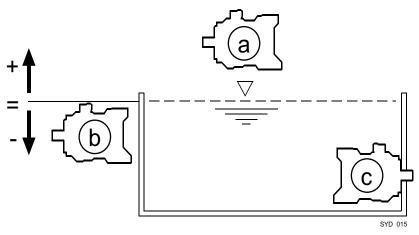
Fig. 18: Installation position
