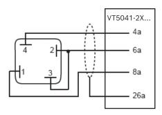
Fig. 25: Connection pattern of the valve position transducer in conjunction with VT5041-2X... (old systems)
