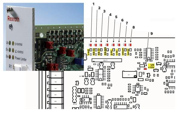
Fig. 36: Fault signals on the printed-circuit board
