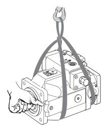
Fig. 17: Transport with lifting strap
