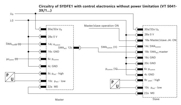
Fig. 14: Circuitry of SYDFE1 for master/slave and independent individual operation
