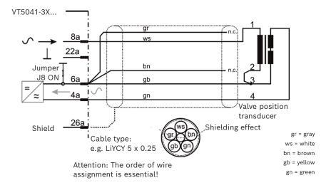
Fig. 26: Cabling for cable lengths up to 50 m
