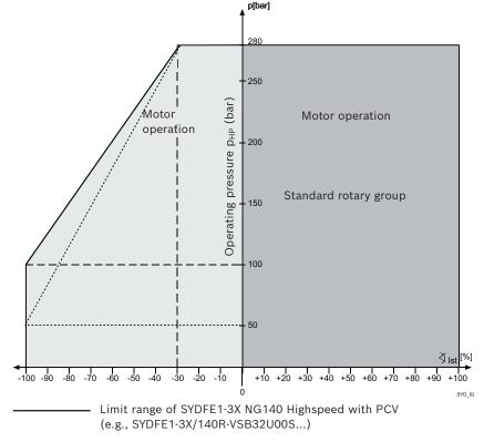
Fig. 9: Operating limits for series SYDFE1-2X and SYDFE1-3X with standard rotary group for brief regenerative operation
