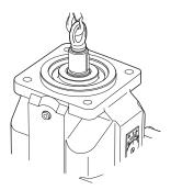
Fig. 16: Fixing the ring screw
