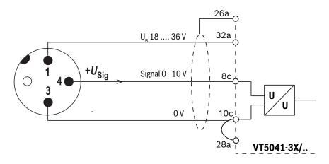
Fig. 24: Connection pattern for pressure transducer HM20...H...
