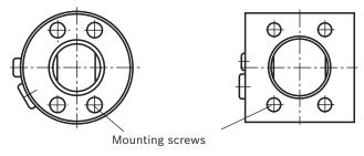
Fig. 34: Mounting bores: left-hand side (round) for NG 18, 28, 25; right-hand side (rectangular) for NG 71, 100, 140
