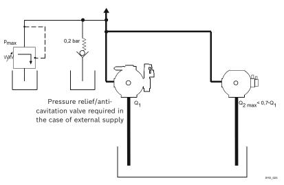
Fig. 7: Circuit diagram for continuous regenerative operation
