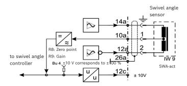
Fig. 28: Connection for swivel angle sensor
