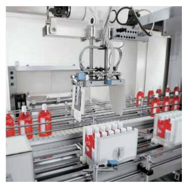
IndraLogic XLC allows you to synchronize up to 64 axes in just one control system, bringing processes into perfect harmony. All processes are transferred to the control system through sercos. The integrated motion logic runtime system considers this immediately when calculating the axis movements. This makes production faster and more precise.
