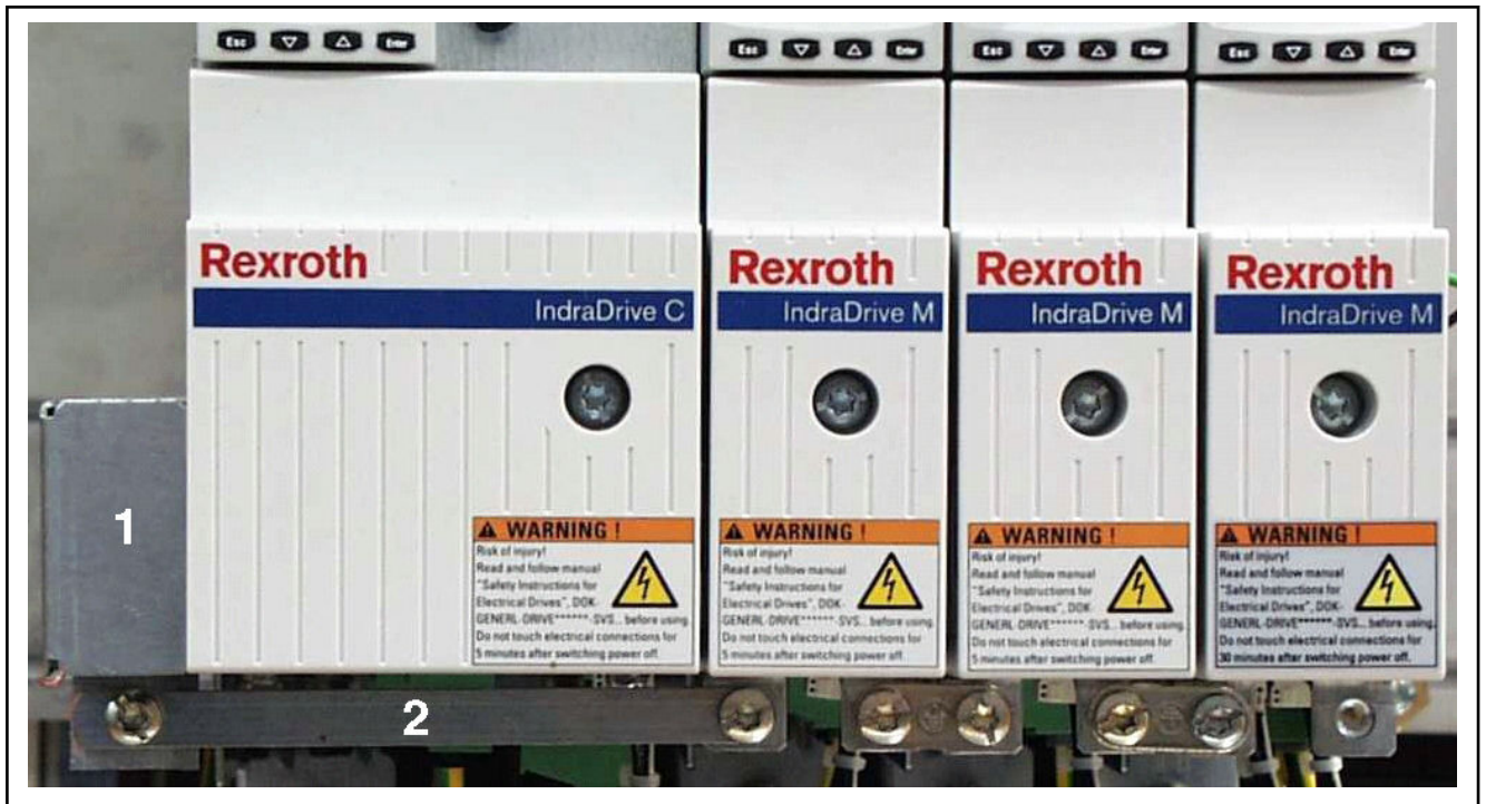
Fig. 20-74: HAS04.1-001 at drive system HCS02 with HMx01 with touch guard mounted
