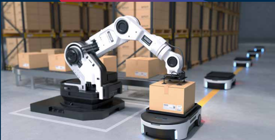
Control system supports automated loading of AGV
